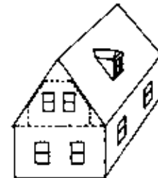
(F) 1 1/2 Story. This type has a high pitch roof with a slope of about \frac{5}{8} or \frac{3}{4} with small dormers on one or both sides of the roof. The area of the finished second floor is approximately 75% of the first floor area.
